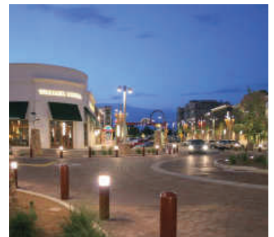
Pedestrian lighting can include fixtures such as bollards, pole lights and accent lighting.
